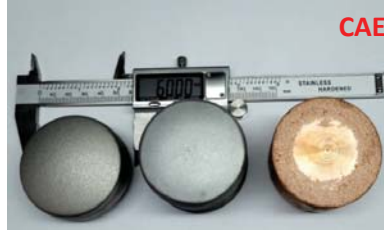
Development of Ti, Cr and Cu coatings by cathodic arc evaporation
